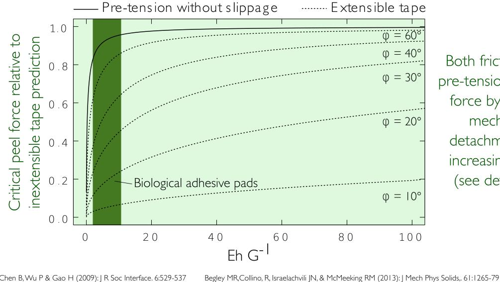
Both frictional dissipation and pad pre-tension increase the critical peel force by reducing the amount of mechanical work done for detachment so that pads behave increasingly like inextensible tape (see detailed leaflet for details).
