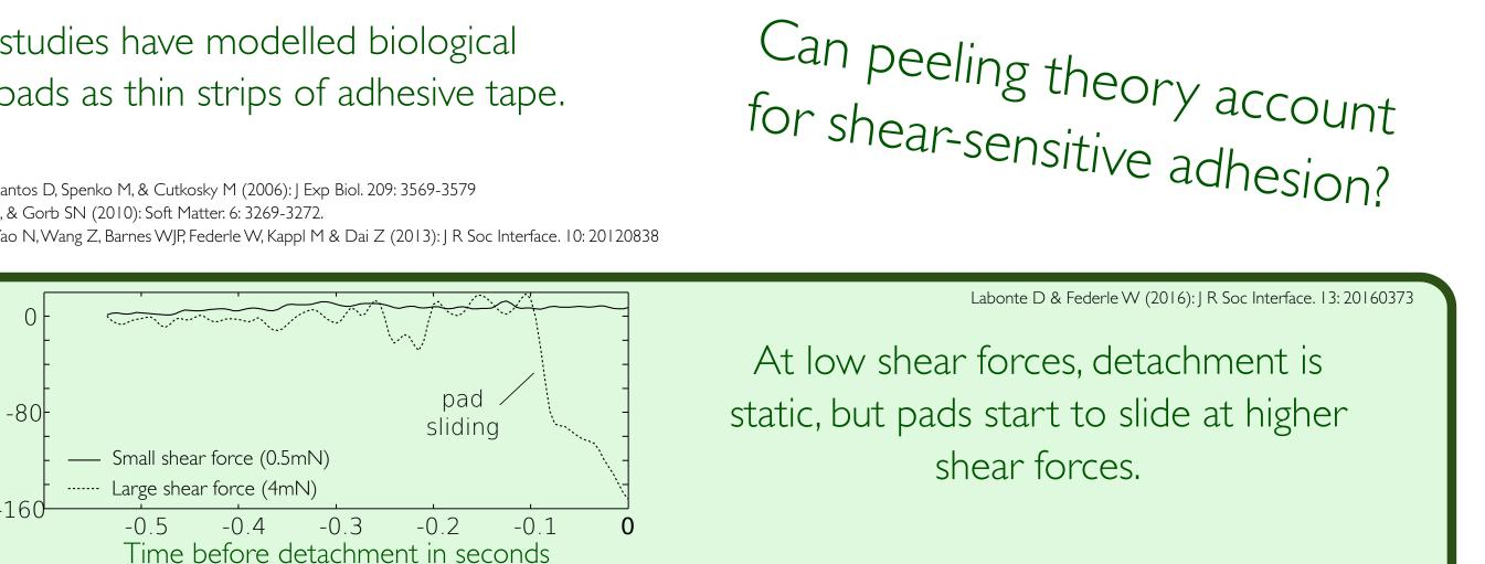
An inextensible tape model works well for small shear forces, but the data are in disagreement with theory as soon as pads start to slide!
