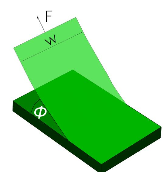
Peeling a unit length of inextensible tape involves work done in creating new surface area, and in moving the point of force appplication. The critical force per unit tape width required for peeling can be found by equating the surface and potential work done:
