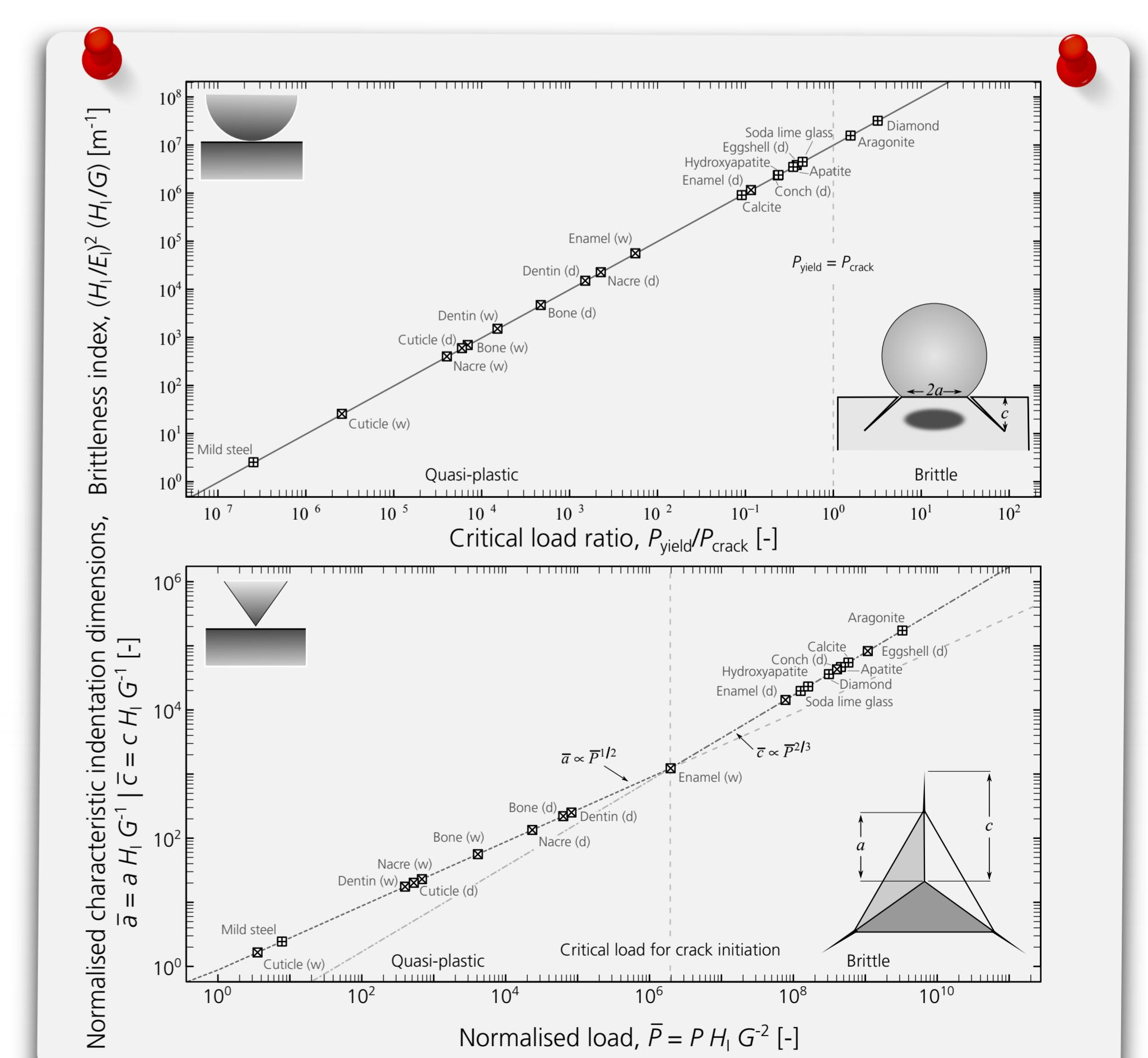
~ Biological materials achieve high toughness via hydration and composite design, at the cost of being more susceptible to quasi-plastic deformation
